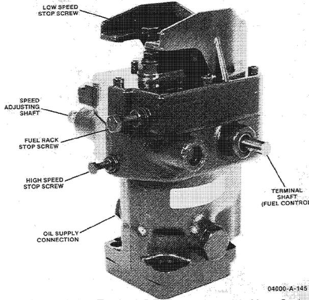
Figure 1-1. Typical SG Governor with New Style Cover
